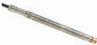
TROLL Shield Antifouling Pressure Sensor Copper pressure sensor nose cone combats biofouling and extends Aqua TROLL 200 and Level TROLL 400/500/700 deployments. #0081480
